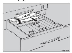
Open the guide under the back guide as shown in the illustration, and then the remove the misfed paper.
